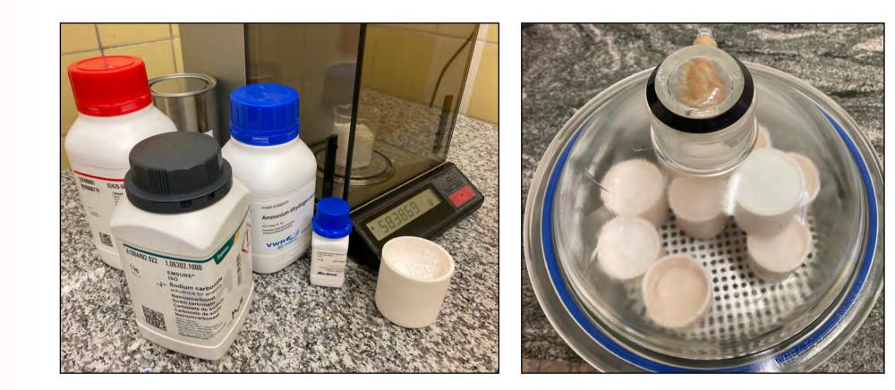
(Left): Raw oxides used for the synthesis of glass, weighed in a high-precision
