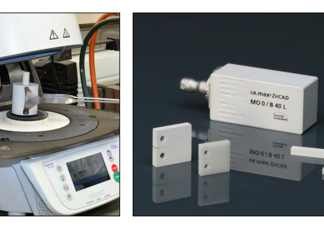
► (Left): Refractory dye inserted containing a glassceramic ingot into a pressing oven.
